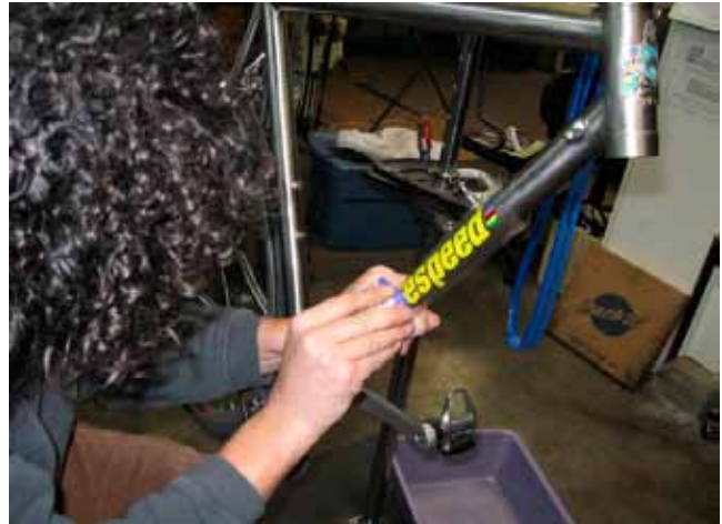
New decal set being applied to brushed finish.
